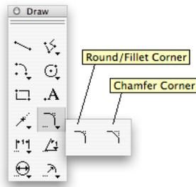
Figure 11.6: Fillet and Chamfer -palette
