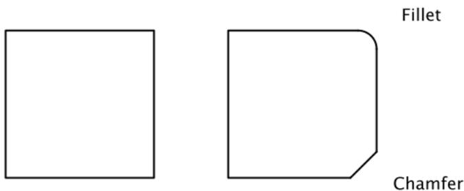
Figure 11.5: Fillets and Chamfers
