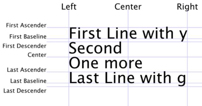
Figure 10.15: Text Block Alignment
