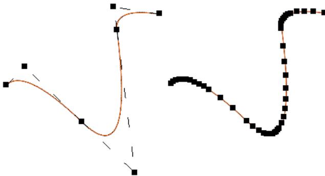
Figure 11.1: Exploding a Spline
