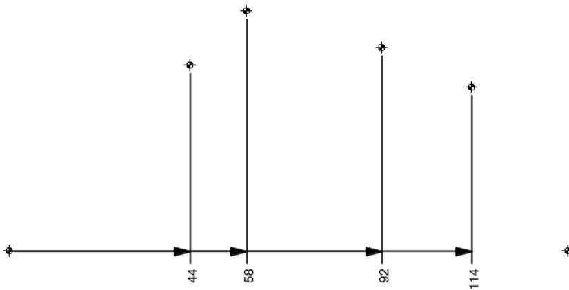
Figure 12.3: Coordinate Dimensioning Example
