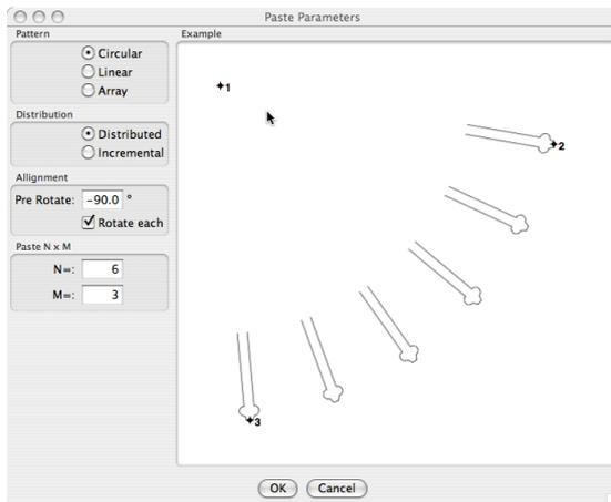
Figure 9.6: Circular Paste Parameters Example
